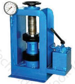
Cube Testing Machine : 05 Nos.
